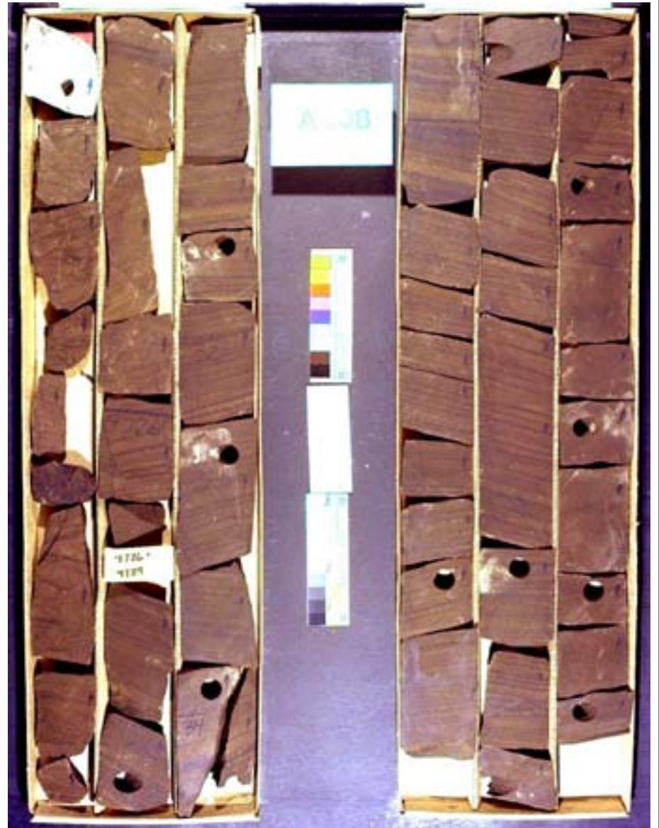
Core from the Upper Minnelusa at the Pan Am 68 Unit Well, showing oil-stained eolian cross lamination. Despite the even stain, differences in permeability among individual laminae may complicate sweep of hydrocarbons to the producing wellbore.
