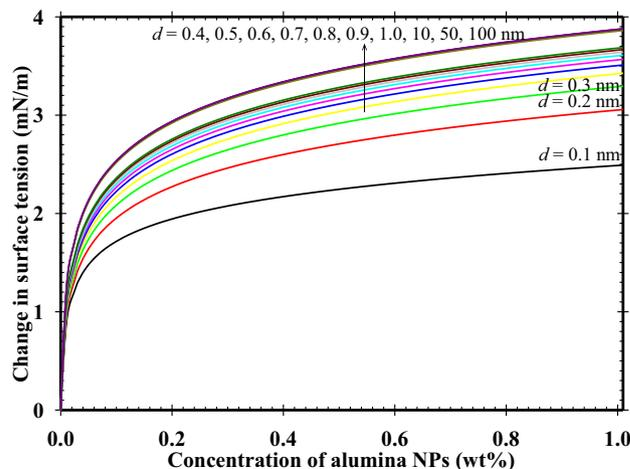
Fig. 7. Type curves for change in surface tension of dispersed alumina NPs in deionized water versus concentration of alumina NPs using the parameters listed in Tables 1 and 3.
