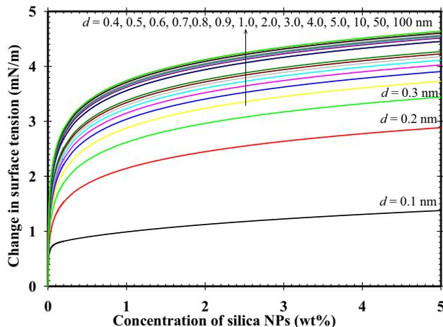
Fig. 6. Type curves for change in surface tension of dispersed silica NPs in deionized water versus concentration of silica NPs using the parameters listed in Tables 1 and 2.
