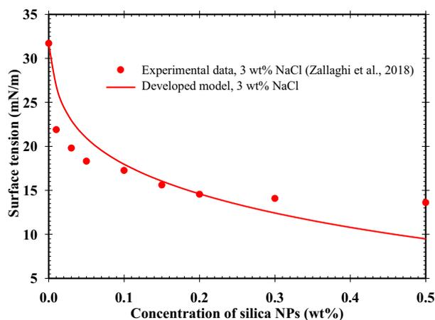
Fig. 4. Surface tension of silica NPs in 3 wt% NaCl solution using the parameters listed in Tables 1 and 5. The results from the proposed model in this study are compared with the experimental data in literature (Zallaghi et al., 2018).
