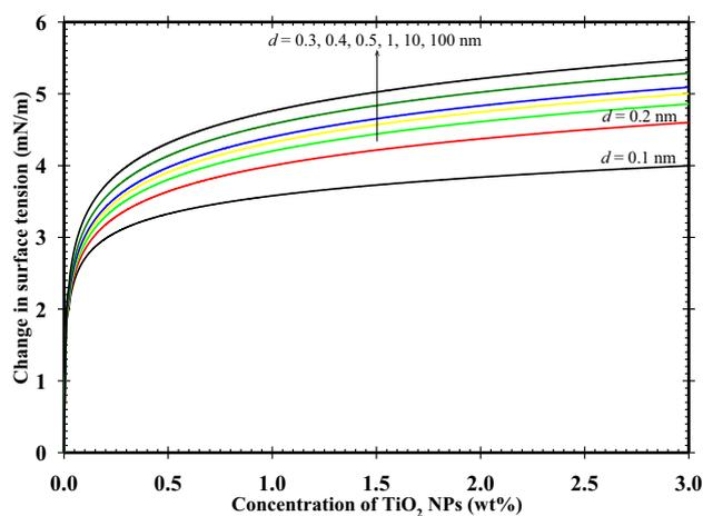
Fig. 8. Type curves for change in surface tension of dispersed  $\text{TiO}_2$  NPs in deionized water versus concentration of  $\text{TiO}_2$  NPs using the parameters listed in Tables 1 and 4.
