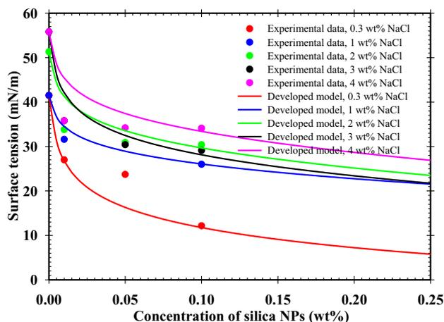
Fig. 5. Interfacial tension of oil-water modifies with different concentrations of NaCl and silica solution using the parameters listed in Tables 1 and 5. The results from the proposed model in this study are compared with the experimental data in literature (Sulaiman et al., 2015).
