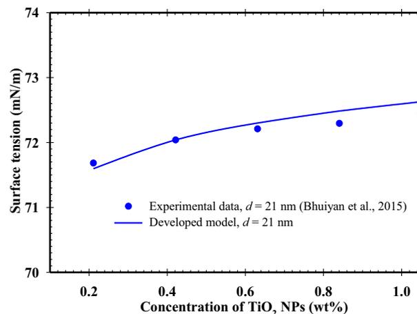
**Fig. 3.** Surface tension of dispersed  $\text{TiO}_2$  NPs in deionized water versus concentration of  $\text{TiO}_2$  NPs using the parameters listed in Tables 1 and 4. The results from the proposed model in this study are compared with the experimental data in literature (Bhuiyan et al., 2015).
