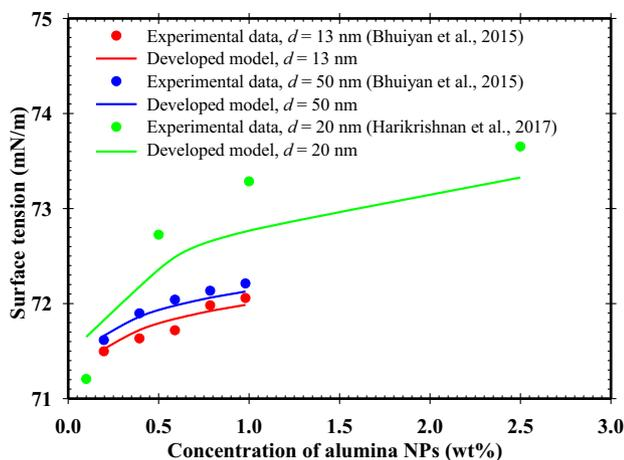
**Fig. 2.** Surface tension of dispersed alumina NPs in deionized water versus concentration of alumina NPs using the parameters listed in Tables 1 and 3. The experimental data used here were reported by Bhuiyan et al. (2015) and Harikrishnan et al. (2017).
