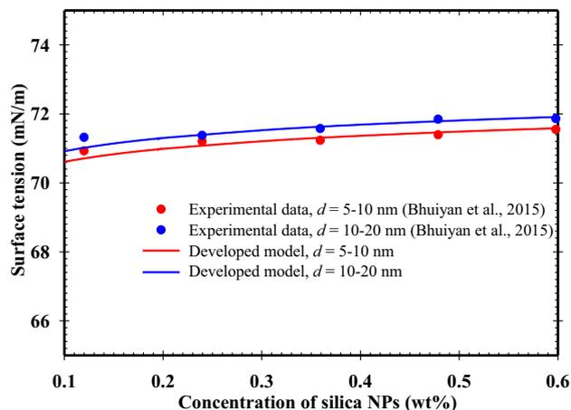
**Fig. 1.** Surface tension of dispersed silica NPs in deionized water versus concentration of silica NPs using the parameters listed in Tables 1 and 2. The results from the proposed model in this study are compared with the experimental data in literature (Bhuiyan et al., 2015).
